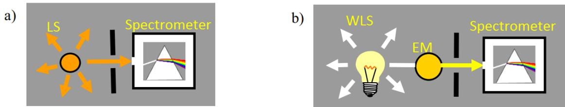
Figure 2: Methods of generating a) emission, b) absorption spectra. Markings: LS - light source, WLS - white light source, EM - examined medium
