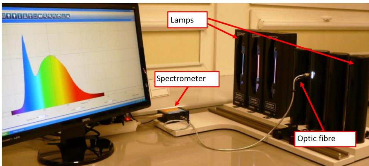
Figure 4: Experimental system used to examine optic emission spectra
