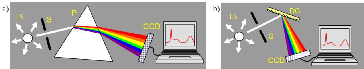
Figure 1: Schematic model of optical spectrometer a) equipped with prism b) equipped with reflective diffraction grating. Markings: LS - light source, S - slit, P - prism, CCD - charge-coupled device, DG - reflective diffraction grating
