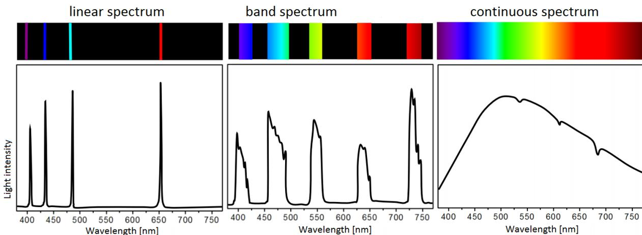
Figure 3: Examples of emission spectra: linear, band, continuous. Top images shows separated rays of light, bottom registered spectra
