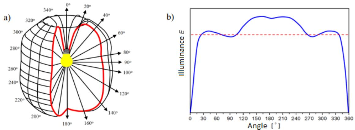
Figure 2: Example of light distribution by light bulb a) candlepower-distribution solid, b) illuminance as function of angle (direction) of emission. Dotted line shows average value.
