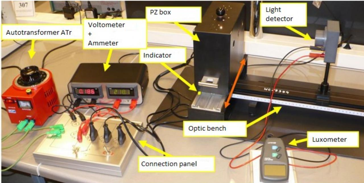
Figure 3: Experimental system used to measure luminous efficacy of selected light sources
