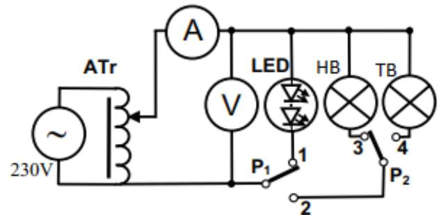
Figure 4: Electric scheme of power system and power measurement
