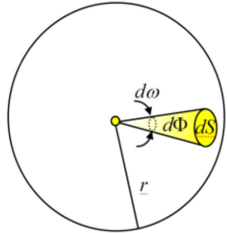
Figure 1: Radiation of point light source
